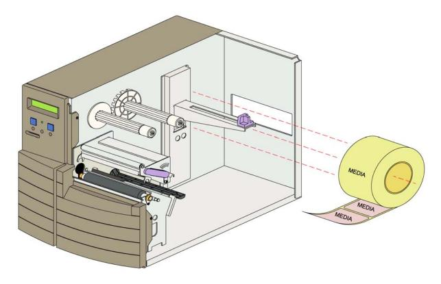
Figure 3-3a, Rolled Media Loading
